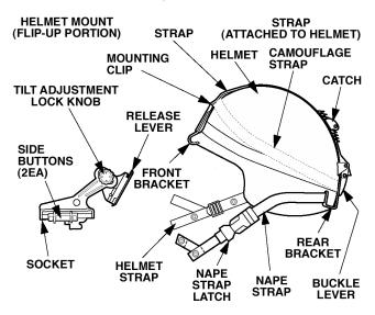
Figure 2-18. Helmet Mount Components and Features.
